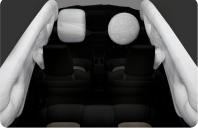
**Dual Front, Side and Curtain Airbags** for protection against side impact
